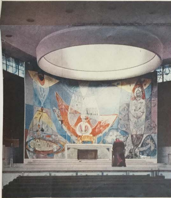
CYLINDRICAL CHAPEL at Massachusetts Institute of Technology uses halo illumination and a screen of metal hung on rods. Designed by Eero Saarinen and Associates, it is 50 feet in diameter. It is surrounded by a moat whose water reflects soft light into the cylinder through arches in its base.
