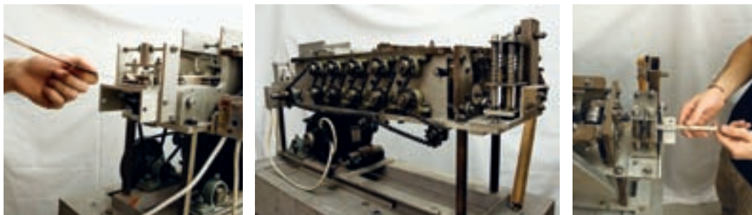
Fig. 32. Machine created by Carlos Cruz-Diez to fold aluminum into U-shaped channels.
