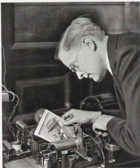
"Captain Richard H. Ranger—Inventor." 1924. "The inventor examining a photograph which has just been made by the receiving equipment following the [radio] transmission of the original photograph. Note the delicate mechanism required at the receiving end." Thomas Coke Knight/RCA.
